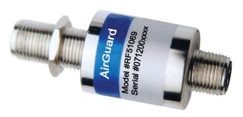
The FGT range of surge protection devices prevents surges and transient overvoltages conducted through coax cables used for wireless Local Multipoint Distribution System (LMDS), Wireless Local Loop (WLL), and Multichannel Multipoint Distribution Service (MMDS). These versatile products can be used in any "F" connector application from DC- 2.5GHz frequencies to 75 ohm impedance.
